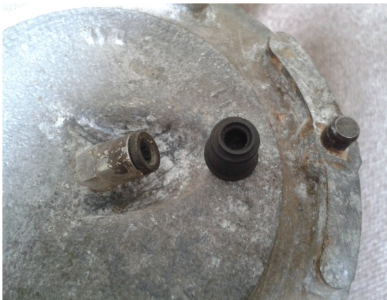
The elusive rubber boot/valve stem oil seal on top of the rear air spring
