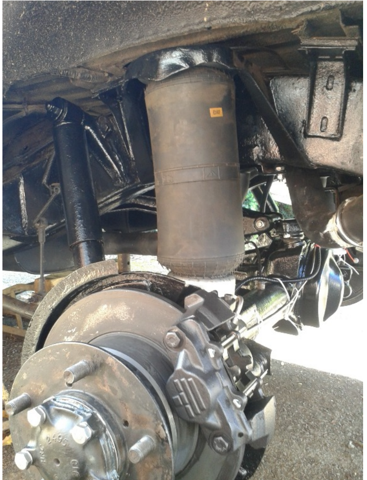
Showing new discs and callipers, new air springs and refurbished shocks.
