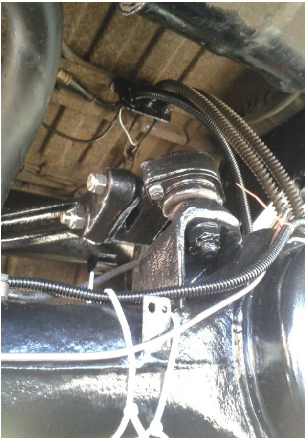
Top Ball Joint. Unfortunately, not a stainless nut as it also has a funny thread.
