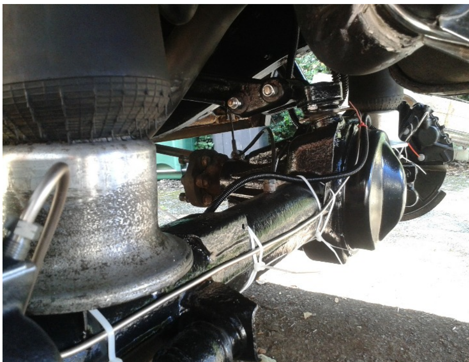
Axle painted and back in position. New brake pipes and wiring.
