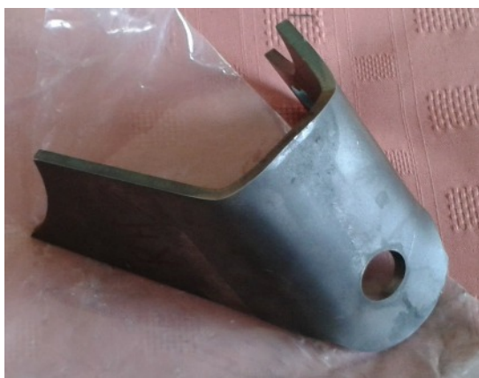
One of the new shock absorber mounts before welding on.
